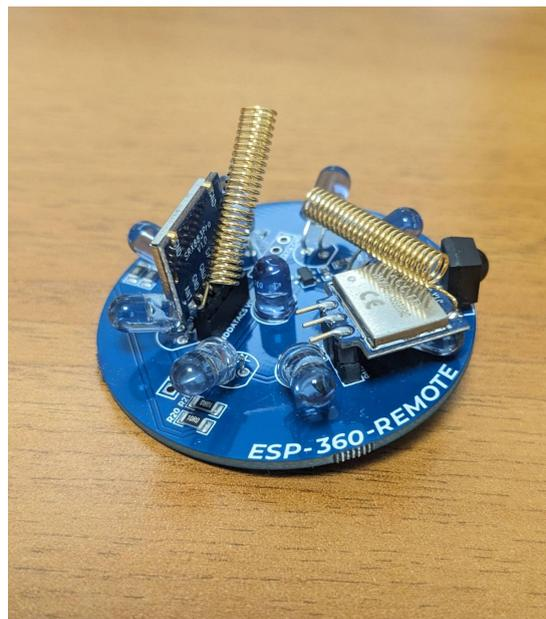
**Step 3:** Insert the top PCB all the way into the base through the 8-pin connector.
