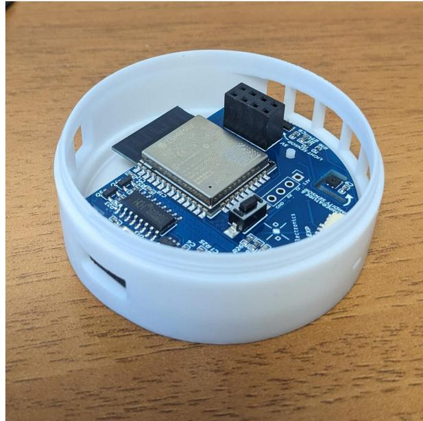
**Step 2:** Insert the RF modules into the upper part of the PCB as shown in the picture and manually raise the infrared LEDs to a 45° angle. They are currently bent horizontally for transportation safety reasons.
