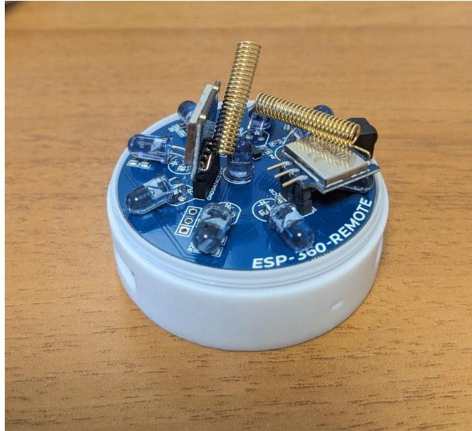
**Step 4:** Close the case by screwing the top part, plug in the power cable, and wait for the board's hotspot called **Esp360Remote** or **Esp360Remote2** (if you ordered the teo pack) to appear!
